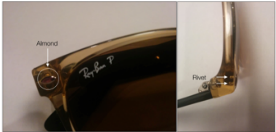
Figure 4. (Left) One of the almonds highlighted in one of the corners of the frame (Right) The same corner of the frame but viewed from above. Note the double-pronged rivet embedded in the nylon polymer frame
